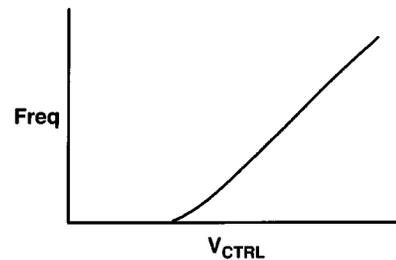
Fig. 10. Typical VCO frequency as a function of control voltage when implemented with symmetric load buffer stages.
