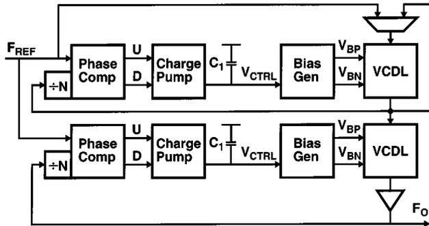
Fig. 17. Dual-loop DLL block diagram.
