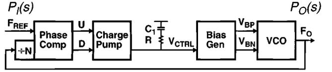
Fig. 9. Typical PLL block diagram (clock distribution omitted).
